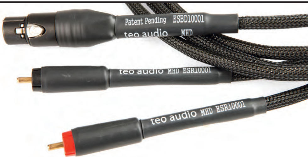
ABOVE: Balanced (analogue and digital – XLRs) and single-ended (Eichmann RCAs) interconnects both use a single 18-gauge core of liquid metal alloy for signal and a copper braid for ground/return (respectively). The plugs are soldered onto barbed copper inserts that make electrical contact with the liquid alloy inside the cable
